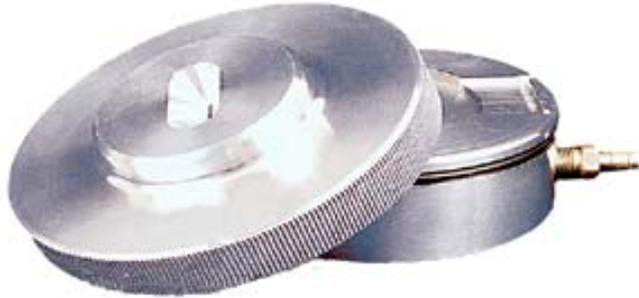
The BioSIS™ was developed as a re-useable bioaerosol sampling device, employing industry standard slit impaction sampling techniques. The BioSIS™ is suitable for the collection of particulates such as mold spores, pollen, skin fragments and other aeroallergens for reliable bioaerosol contamination studies. The improved venturi design creates laminar flow for more defined impact zone allowing precise analysis. The BioSIS™ can be calibrated for more accurate results. Other features include:
