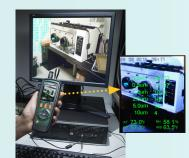
Particle Counter with unique built-in camera for capturing videos and photos that are stored onto internal memory or a microSD card. The VPC300 can measure up to 6 channels of particle sizes plus Air Temperature and Relative Humidity. Use the included software to generate reports with videos, photos, and data points.
