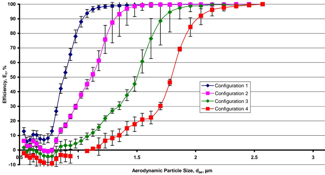
FIGURE 2. EMS IMPACTOR EFFICIENCY FOR DIFFERENT CONFIGURATIONS MEASURED WITH **OLEIC ACID PARTICLES** AT 20 LPM.
