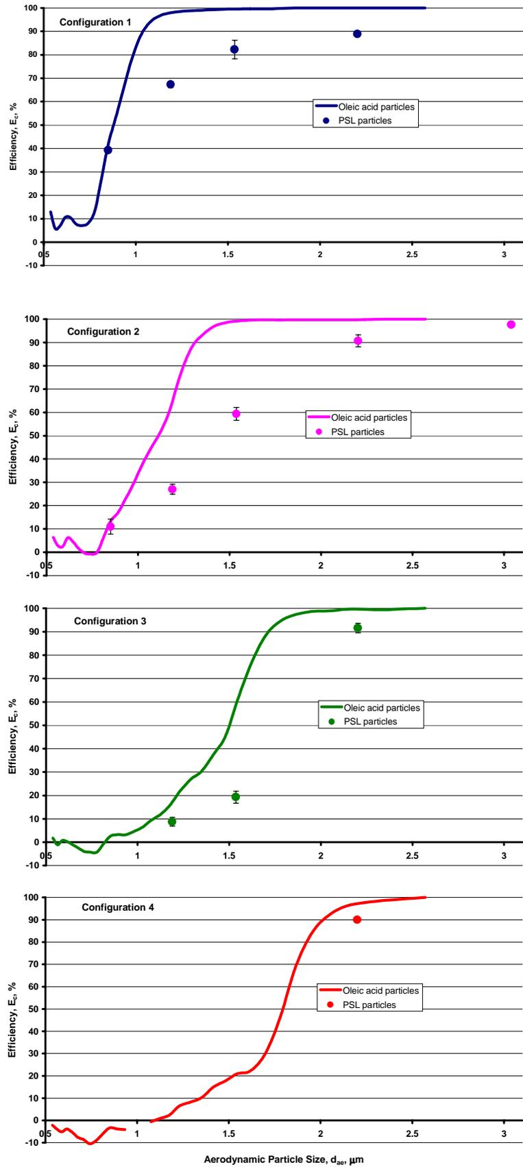
FIGURE 3. EMS IMPACTOR EFFICIENCY FOR DIFFERENT CONFIGURATIONS MEASURED WITH OLEIC ACID AND PSL PARTICLES AT 20 LPM.
