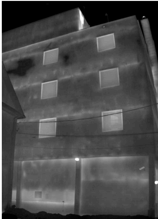
Figure 12. Negative Building Pressure (-140 Pa), T_o = 0^\circ\text{C}
