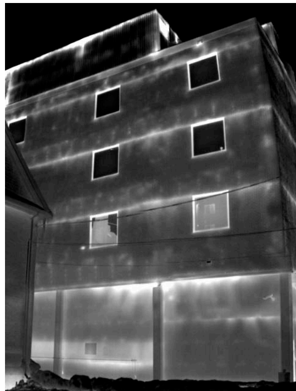
Figure 16. Positive Building Pressure (+25 Pa), T_o = -11^\circ\text{C}
