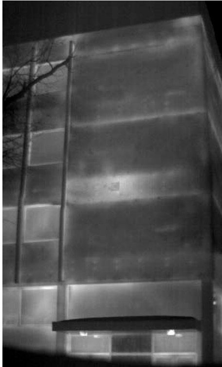
Figure 6. Negative Building Pressure (-140 Pa), T_o = 0^\circ\text{C}
