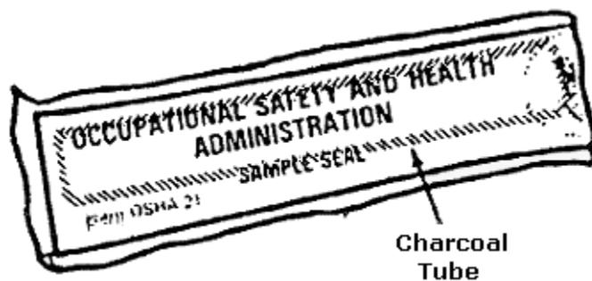
**FIGURE II:1-4b. INCORRECTLY SEALED C-TUBE. END CAPS CAN BE REMOVED AND SAMPLE INTEGRITY JEOPARDIZED WITHOUT DISTURBING THE SEAL.**
